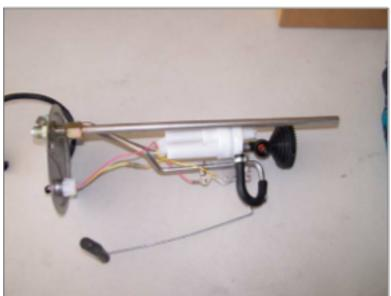
Secure the pickup tube to the bulkhead fitting as shown.
