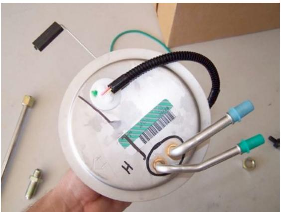
We recommend the use of a stepped drill bit for drilling the sending unit plate, these typically result in the best quality hole. The hole should be drilled just large enough for the bulkhead fitting to fit through without leaving too much gap around it.
