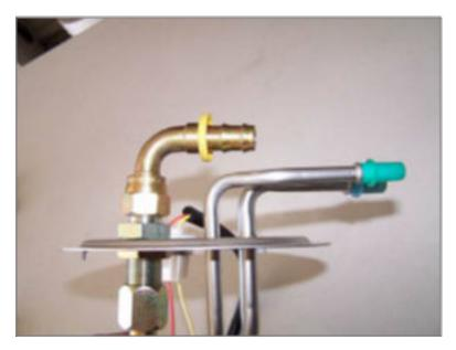
Installation of this fitting requires some muscle. We recommend keeping the fitting cool and the hose warm until you're ready to work with them. It is sometimes beneficial to put the end of the hose into a bucket of hot water just prior to installing the fitting as this helps to soften the hose temporarily, making it easier to work with.
