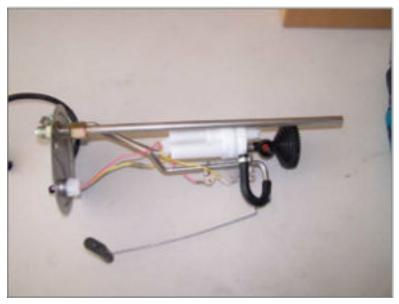
Secure the pickup tube to the bulkhead fitting as shown.
